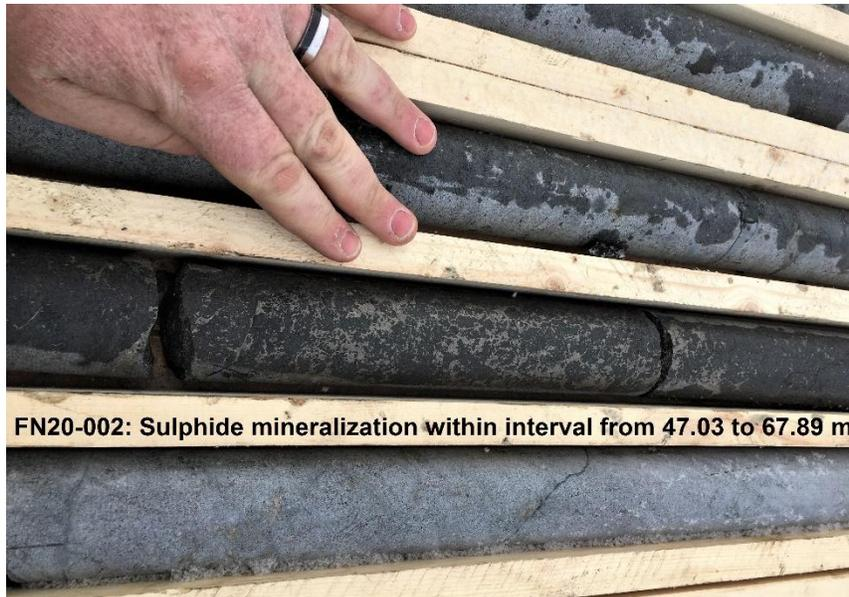
ALX’s first hole, FN20-001, was drilled to a depth of 165 metres but did not encounter significant sulphide mineralization. A borehole electromagnetic (“EM”) survey was immediately carried out upon completion of the hole, which detected a conductive zone at a shallower depth. Hole FN20-002 targeted this anomaly from the first drill set-up. A comprehensive ground EM survey is recommended over V-1 to better define conductive zones in the V-1 area, when ground conditions permit.
