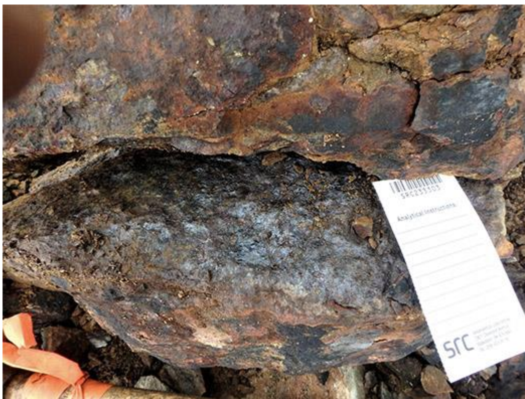
Close-up of sample from historical trench at Conductor 6-D (1.11% Ni, 0.42% Cu)
